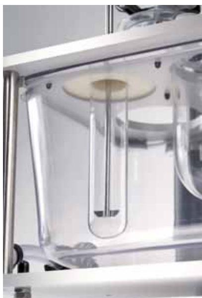
708-DS conversion kit, 200 mL vessel with mini paddle
