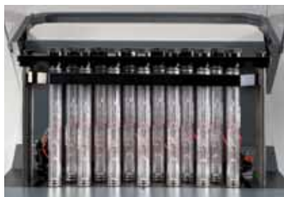
Internal view of cell holders
