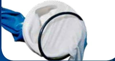
**Step 5** Place new glove into the sleeve.
