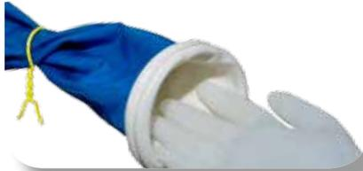
**Step 6** Fold glove over cuff ring and install spring.
