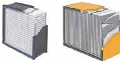
Esco cabinets use Swedish Camfil Farr® mini-pleat filters without aluminum separators to increase filter efficiency, minimize the chance of leakage, and to prolong filter life. Filters include a lightweight aluminum frame for structural stability and elimination of swelling common to conventional wood frames.
