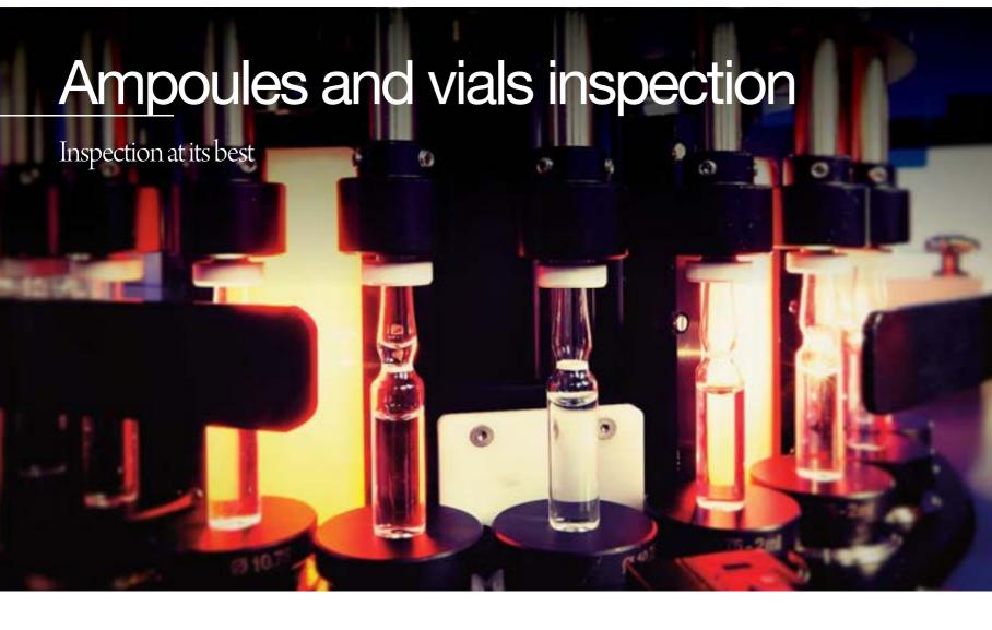
CMP inspection machines by TV cameras and magnifying lenses:
